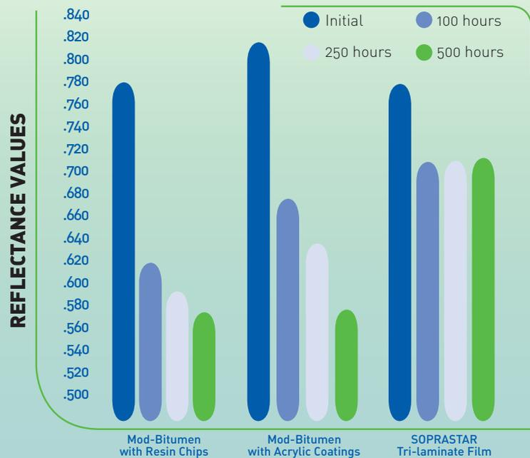
Reflectance is the proportion of light that a surface reflects compared to the amount of light that falls on that surface. The color black has a reflectance value close to zero while white has a reflectance value of nearly 100, which keeps a building light and cool. All colors fit between these two extremes (called the start value).
