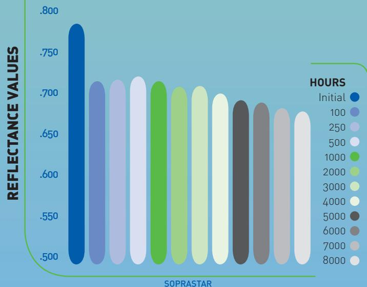
\* The information contained in this brochure has been verified in SOPREMA's own and/or independent laboratories; based on ASTM 459 4 hours.
